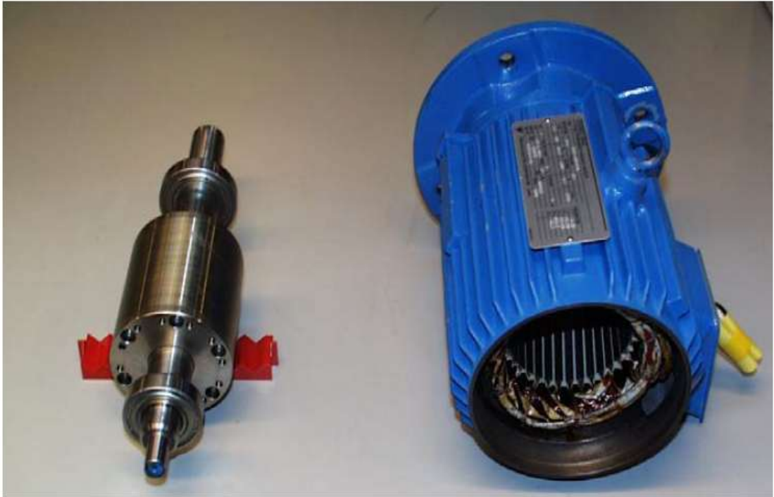
A1.1. View of rotor (on the left side) and stator armature (on the right side) of PMSM.
